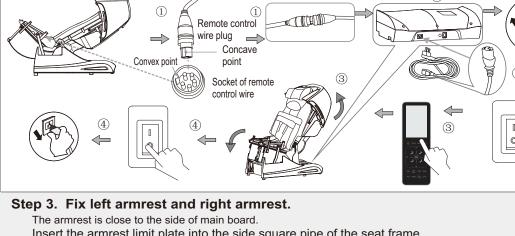
Insert the armrest limit plate into the side square pipe of the seat frame.
